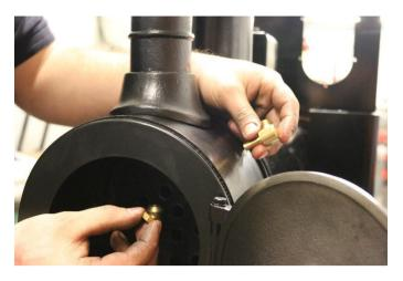
Fit smokebox steam blower fitting through the smoke and lock into place with the nut.
