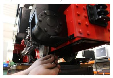
Put the two M3 x 5 button head screws in the underside of the cylinder for the cylinder cladding, leaving them loose to slide the cladding sheet in.
