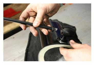
Screw the dummy regulator rod in to the regulator and lock off the nut.
