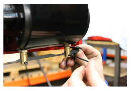
Endo the securing screw ensure that you keep the operating rod in place (if this drops out of place the small dowel will drop out). Fit the operating rod in to its locating hole and retighten the securing screw.
