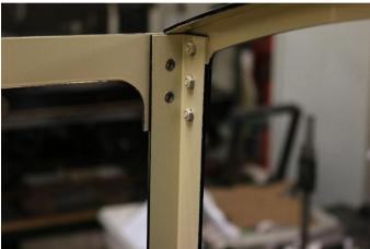
Assemble the rear cab support using M4 x 10 Hex Head bolt and nuts. Assemble onto the engine and bolt into place using M4 x 10 Hex Head bolts and nut at the top and M6 x 10 with washer on the bottom, this is fixed from the underside of the footplate and screws into the support base plate.
