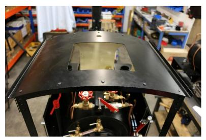
Cab roof can then be fitted at this point. This is secured in place using eight M4 x 10 hex head bolts.
