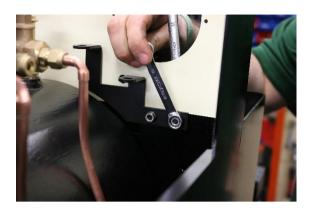
Fit the pressure gauge bracket using M6 x 12 hex head bolts with turned down head (3mm thick). Ensure that the head of the bolt is threaded throw the cab from the outside of the cab, this ensure clearance on the water tank when we come to fit them.
