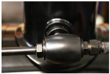
Before fitting the steam dome you will need to fit the dummy regulator and dummy Safety valves, all of which are bolted up from the inside of the dome. For the dummy safety valves use M8 x 20 hex head bolts and for the dummy regulator use a M6 x 20 hex head bolt.
