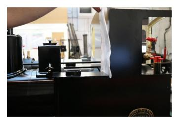
Fit Tanks into there outer pockets. Use a peace of paper at the back of it when fitting as this will prevent scratching the paint work.
