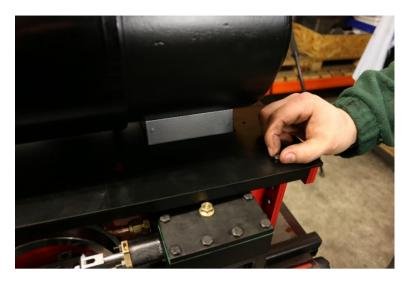
Fit the front decks, these just slot Into place and bolt on at the front using two M4 x 10 hex heads.
