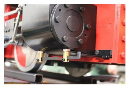
Fit the drain cocks to the cylinder lining the two up so as they run in line with one another. Loosely fit the operating rod to ensure that they are in line.
