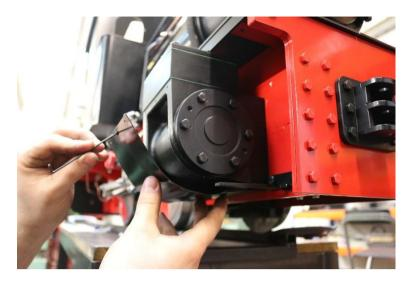
Slide the cladding on to the bottom two screws. Then fit the centre top screw in and screw on to the cylinder.
