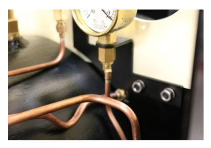
The ejector exhaust is threaded throw the square hole just under the pressure gauge bracket. This is a fiddly job as you have to weave it throw the per-fitted pipe work.
