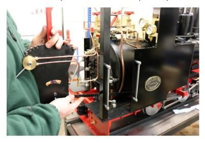
Fit on the reverser level assembly. This is easier to fit up in one peace (including the Vac Brake valve pipework) as it save's a lot of the fiddly fitting after.
