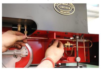
Fit the water tank to water valve pipe work and tighten up the compression fitting.
