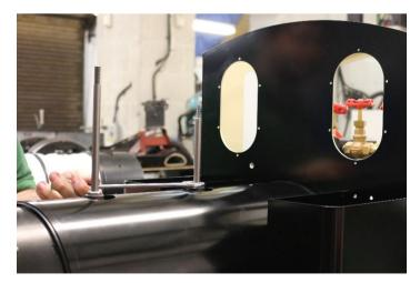
Both the Sand and steam dome studs are fitted at this point, the longer one of the two is for the steam dome and is fitted nearest the front of the engine. They are supplied with an M10 lock nut and they simply screw into the bushes and lock the nut off to ensure a secure fixing.
