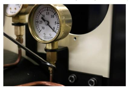
Connect the Vaccum gauge pipe work to the Vaccum Gauge.
