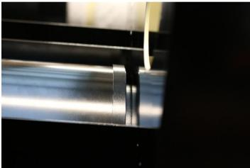
The rear boiler band is the next to be fitted, this is fitted over the boiler and slide back towards the cab till it is flush with the boiler cladding. Access to the tabs is from the underside of the water tanks. This can be tricky and help of an extra per of hands my by useful. Please note that the middle boiler band doesn't go on at this point, it is best to fit this after fitting the dummy sand and steam dome to ensure that it is seated mid-way between the two.
