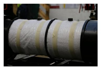
Wrap boiler lagging around the boiler and secure in place with masking tape.
