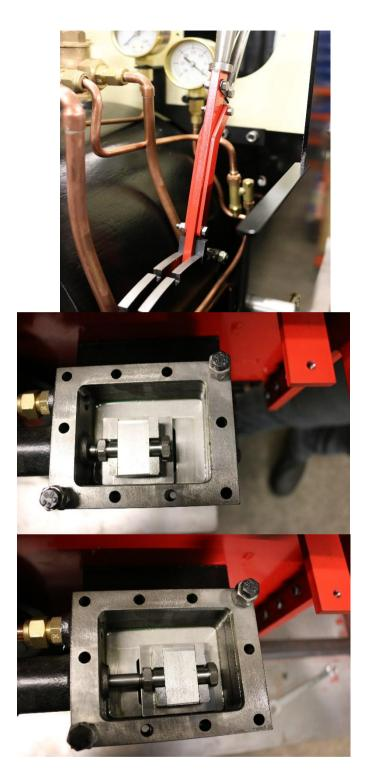
To set the valve gear take off the valve chest cover plates and set the reverser to the first notch forward. Roll the engine forwards and backwards adjusting the slide valve locking nuts until there is an equal valve opening on both sides.
