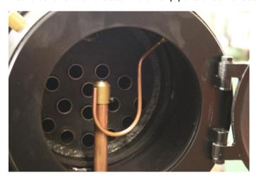
Finally fit the blower pipe to the tail of the smokebox fitting inside the smokebox.
