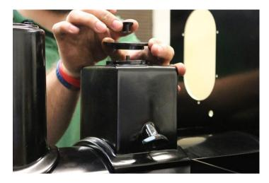
The dummy sand dome is then fitted on to the engine, this is secured by using the lid and the knob to fasten the dome down. Once the lid is in place apply some 243 loctite to the threads on the knob and secure into place.
