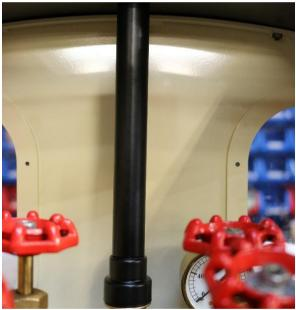
Fit the safety valve chimney, this simple fits through the cab roof and seats back down on to the top of the safety valve.
