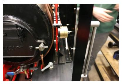
Bolt it in to place with M6 x 10 Hex head bolts with washers.
