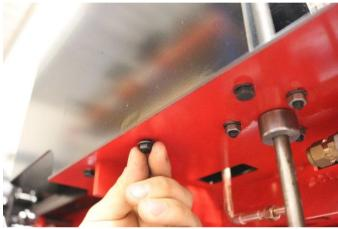
With the help of a friend lift the cab into place and bolt down using M6 x 10 Hex head bolts and washers.
