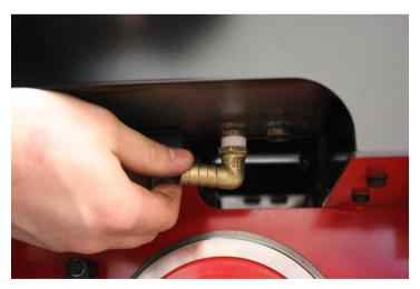
Fit the 3/8" BSP brass hose tails to the underside of the tanks use PTFE tape to seal. The hose tail should be facing in towards the frame when fitted.
