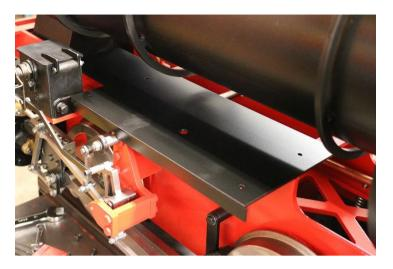
Fit the Left and the Right side rear decks to the chassis and bolt into place using M5 x 10 Hex head bolts.
