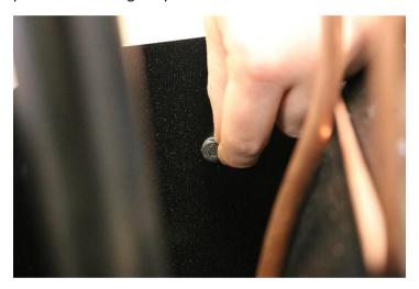
Bolt the tanks in to place from the inside of the cab using two M6 x 12 hex head bolts and washers.
