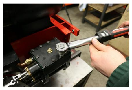
Put the valve chest cover back on and bolt down. All bolts should be torqued down to 13 NM.
