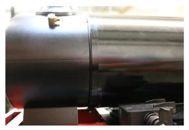
The boiler cladding is then held into place with the boiler band and these are secured by using M4 x 30 Cap Head screws and a nyloc nut. Ensure that the tabs are face under the boiler barrel to hide out of view.
