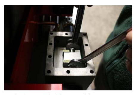
Once the valve gear is set lock of using two 9/16" AF spanners.
