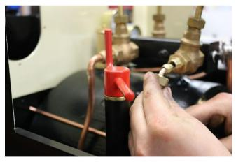
Thread the steam blower pipe through the square hole in the spectacle plate and fit to the steam valve on the fountain.
