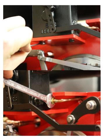
Fit Lubricator to the mounting Bracket Using M4 x 10 Hex head bolts. Fit lubricator pipe to the union and tighten.
