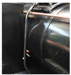
The dummy sand dome pipes fit through the hole in the decks and then fix's to the 8mm compression fitting on the dummy sand dome.
