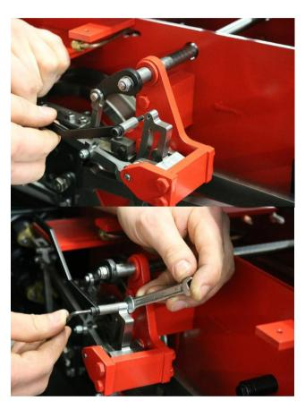
Fit lubricator link arm using using a M4 x 35 Cap head with a 17mm spacer and bolt to the top threaded hole on the expansion link (10101), Finally secure using an M4 nyloc nut on the back side of the expansion Link.
