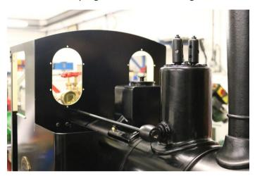
To fit the dummy steam dome you we need to seat it over the mounting stud threading the dummy regulator rod through the hole in the cab first before finally seating it onto the boiler barrel.
