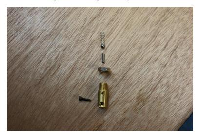
The assembly of the drain cocks is as shown in the above picture. Pre-assemble all the drain cocks.
