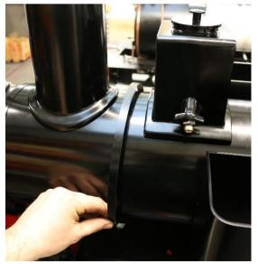
The last of the three boiler bands can now be fitted. Ensure that the band if sat mid-way between the sand and steam dome before the final tighten.
