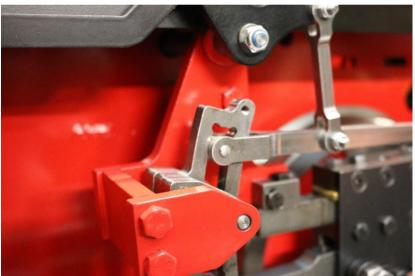
To determine where the reverser sits the return crank needs to be set at approximately 45 degrees (as shown in the above picture). Adjust the position of the reversing stand until the gap at the top and bottom of the expansion link to die block is equal. Once this is equal top and bottom bolt the reversing lever stand in its final place.
