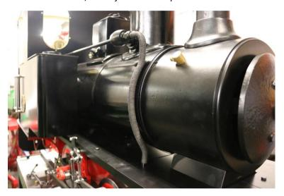
Fitting the dummy steam pipe simply fit through the hole on the deck and is tighten in to the 10mm compression on the dummy regulator.
