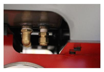
Fit the 8mm compression fitting it to the tank, again us PTFE to seal.
