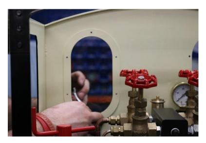
Fit the spectacles starting with the outer one first with two M4 x 10 hex heads ready in place top and bottom. Then place in the glass follow by the inner spectacle (an extra per of hands maybe helpful at this point). Fit the remaining bolts, don't over tighten the bolts as this could course the glass to crack.
