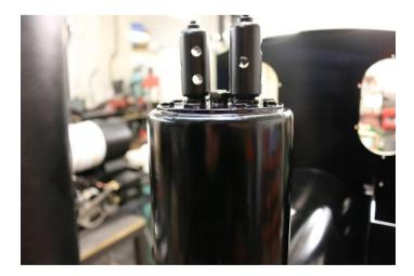
Finally secure down with a M10 lock nut.
