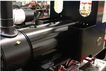
Place on the Boiler cladding starting with the bottom sheet first. This is place on from the top and rolled around the boiler to sit at the bottom. The top sheet then goes on and overlaps the bottom sheet ensuring that the holes line up with the boiler bushes.
