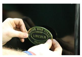
Fit works nameplates to the sides of the cab (holes pre-drilled). These are fixed into place using  $\,$  M3  $\,$  x 12 Button head screws and nyloc nuts.
