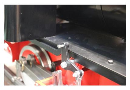
Bolt the reach rod to the reach rod lifting arm using a 20mm motion pin.
