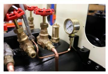
Fit the pressure gauge syphon to the fountain and the pressure gauge.
