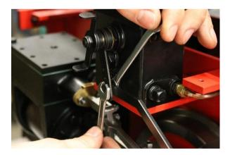
Fasten the other end of the Lubricator link arm to the lubricator using a M4 x 10 Hex head bolt and Nyloc nut, tighten till it nips up then back off half a turn.
